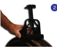
Press down firmly until the tablet holder is located as far down as it can be onto the flywheel.
